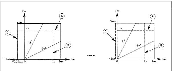
Figure 5-2. Typical Power Supply Operating Curve
